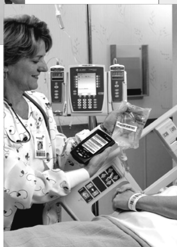
3. Nurse scans IV bag, prompting the transfer of information from the pharmacy directly to the pump.
